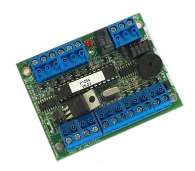
The PACOM 1064 Door Controller Module is a single card reader access control interface designed specifically to operate with PACOM Controllers and security software.
