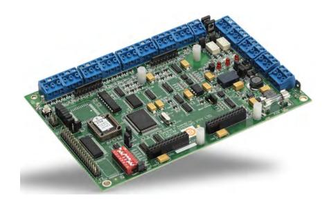
The PACOM 1065 Input Output (I/O) Module is used to expand the supervised alarm input and output points of any of the PACOM Controllers - 8002 or 8003. The module provides 16 supervised input points and 4 output points.
