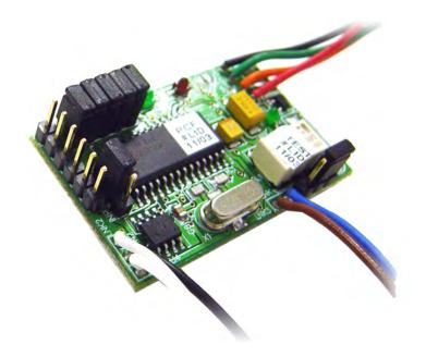
The PACOM 1068 Input Output (I/O) Module is designed to increase the security of remote alarm input devices such as PIR detectors, door contacts and seismic detectors. It is small enough to be housed inside the casing of most devices and has 2 inputs to allow monitoring of the device contact and an additional tamper switch.
