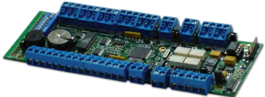
The PACOM 1076 2-Door Controller (DC) Module is a dual card reader access control interface designed specifically to operate with PACOM Controllers and security software.
