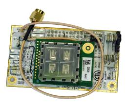
The PACOM 8201 3G Expansion Module enables bi-directional communication between PACOM security software and PACOM Controllers across 3G mobile networks. It provides wireless communications for alarm monitoring, access control operations and system management.
