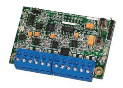
The PACOM 8207 RS485 Star Coupler Expansion Module enables RS485 cabling in a 'star' configuration with up to 4 paths, allowing a maximum of 32 devices to be connected.
