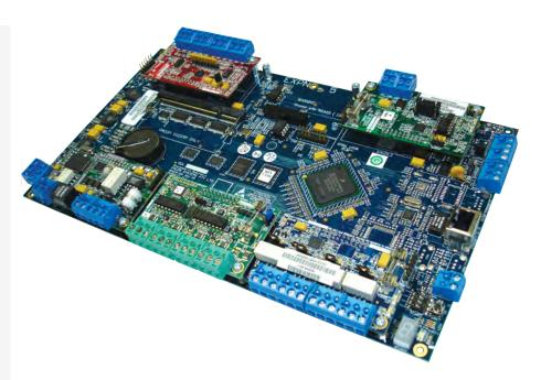
The PACOM 8000 Series Expansion Cards conveniently plug into the controller as 'piggy-back' modules and use the controller as their power source. The modules are automatically configured and the firmware is updated when fitted on the controller or the peripheral device.
