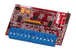
The PACOM 8204 8-Input Expansion Module is used to extend the number of alarm input points to provide 8 supervised alarm inputs. All inputs can be configured for analog operation (0 to 8VDC) when used with the 8002 Controller. The inputs can report the following states: alarm, open circuit, secure/reset (normal), short circuit, trouble/tamper, masking alarm and range reduction.
