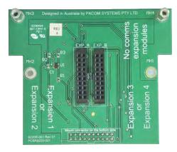
The 8220 Dual Expansion Module is designed to increase the available functionality of the PACOM 8003, 8501 and 8603, connecting up to 4 expansion cards to a single controller/device.
