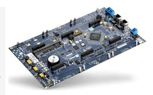
PACOM 8002 next generation controller is built using PACOM-Edge technology. PACOM-Edge represents a new family of devices enabling advanced security capabilities across an organization's Ethernet backbone. The IP capability means there is a reduced need for traditional security cabling which ensures convenient deployment and extensive scalability.
