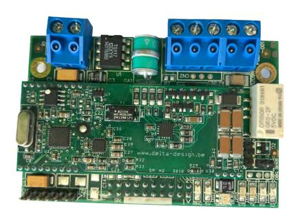
The PACOM 8209 PSTN Modem Expansion Module is designed to provide a backup communications option for the 8000 Series PACOM Controllers across a PSTN line.
