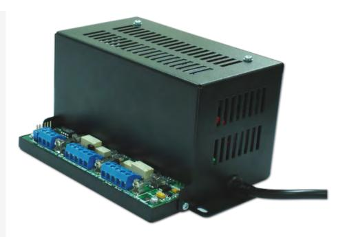
The PACOM 8303 Monitoring Power Supply provides a regulated 12 to 15V DC supply for powering controllers, peripheral devices and charging backup batteries. The power supply unit can be remotely configured, controlled and monitored by PACOM security management software. A PACOM Controller acts as an interface to the 8303 via RS485.
