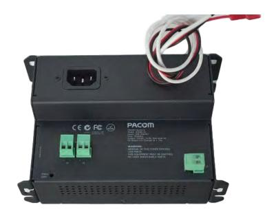
The PACOM 8309 Power Supply Unit (PSU) provides a regulated 10.5 to 17.5 VDC supply for powering controllers, peripheral devices and charging backup batteries. It can be remotely monitored by PACOM Security Managment Software. A PACOM Controller acts as an interface to the 8309 PSU via the status wire.
